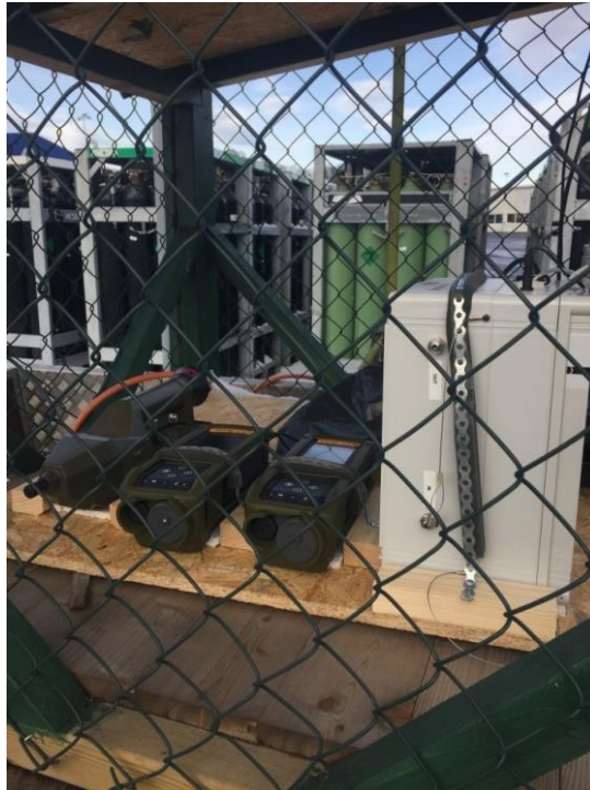
Figure 2 – EU-SENSE node setup during outdoor measurement session in Norway (source: FFI)
